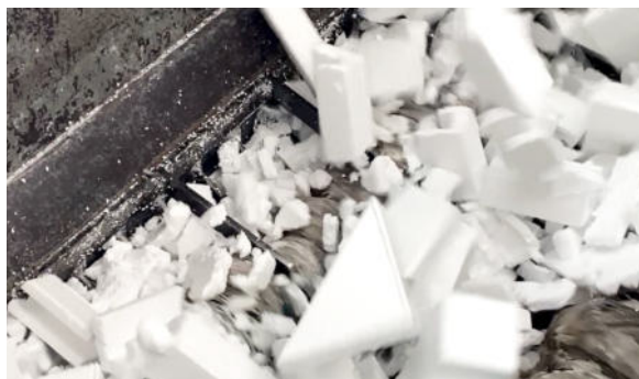
The polystyrene is crushed to obtain much coarser pieces
