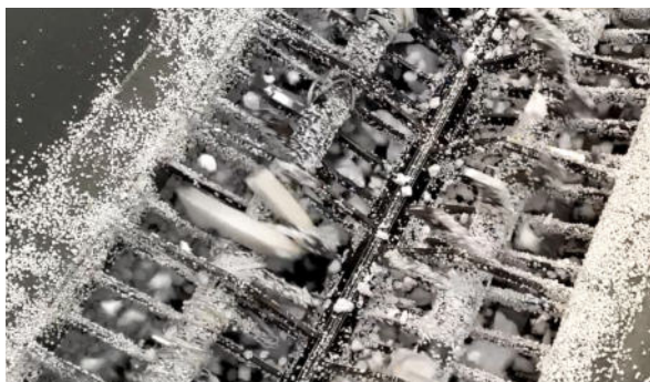
The EPS is ground in order to obtain very fine pieces
