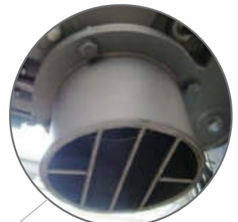
Unloading port with manual opening and safety grid
