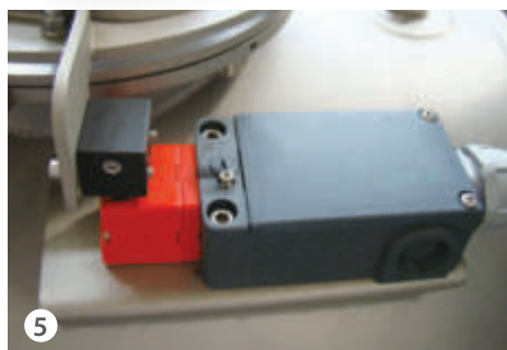
5 Accident-prevention electric lock
