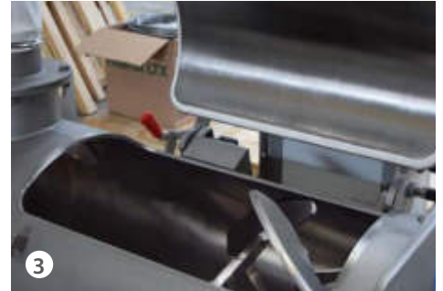
3 Loading and inspection hatch with safety block
