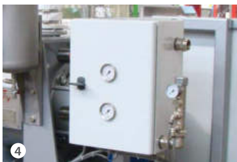
4 Pneumatic control panel
